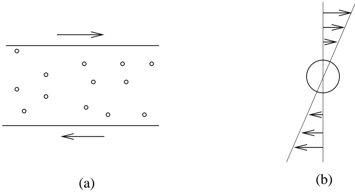
Figure 9.4: Shear flow of a suspension (a) and the shear flow around a particle (b).
