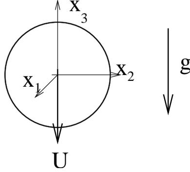
Figure 9.3: Sphere settling in a fluid.
