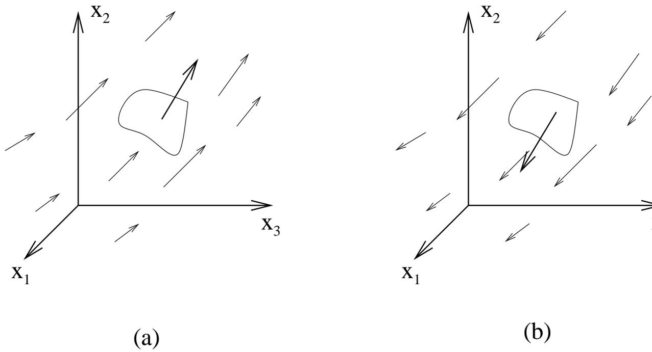
Figure 9.1: When the force exerted on the fluid is reversed, the fluid velocity is reversed at all points in Stokes flow.
