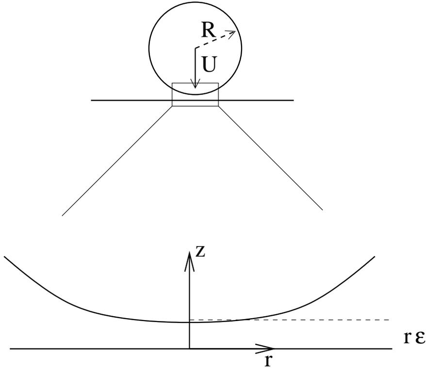
Figure 9.5: Lubrication flow in a small gap between a sphere and a solid surface.
