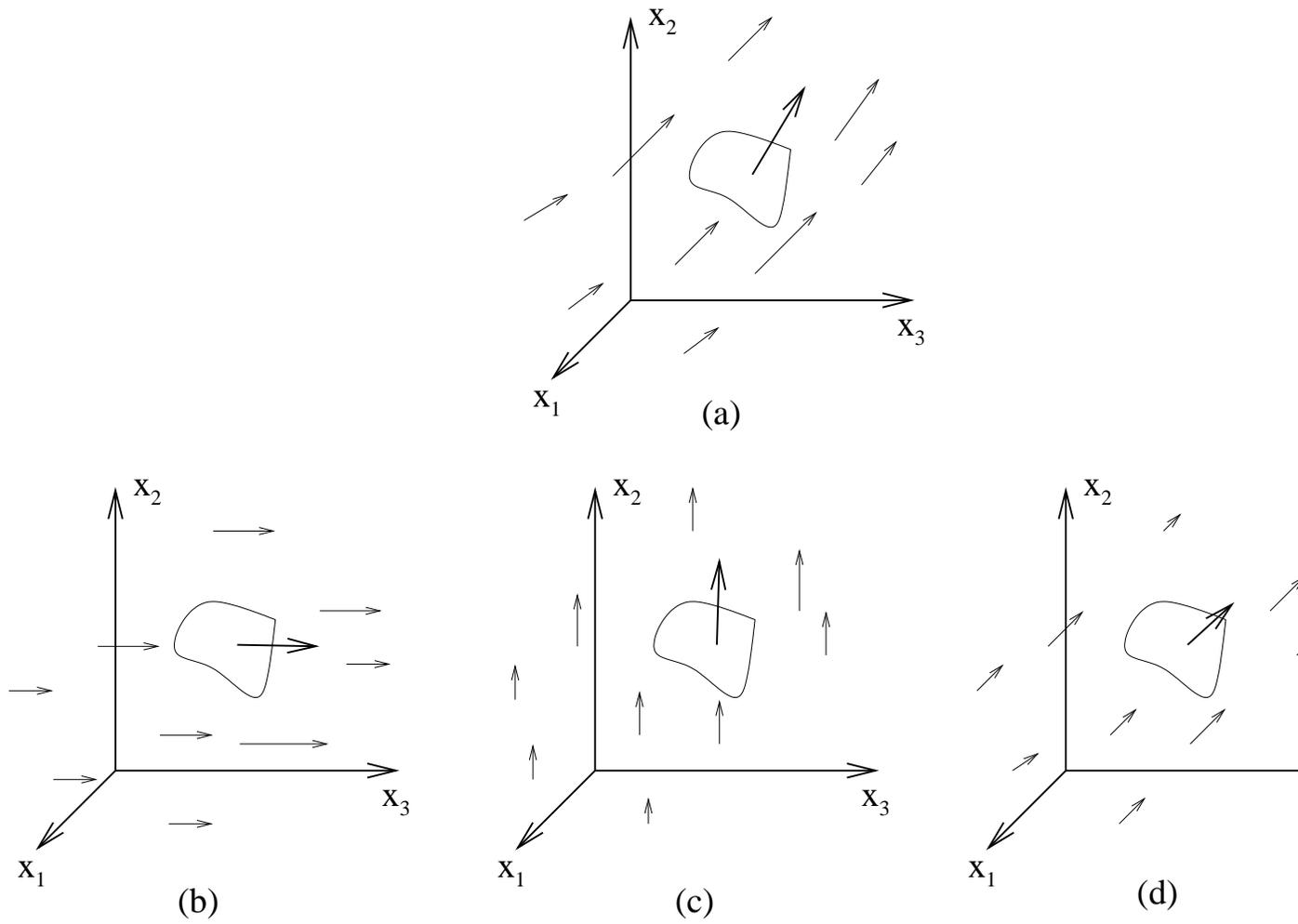
Figure 9.2: Use of linear superposition for separating the problem into simpler sub-problems.
