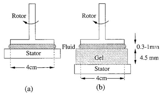
FIG. 4. Rheometer used in the experiments: (a) unmodified; (b) modified.
