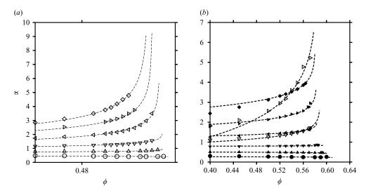
FIGURE 4. The parameter  $\alpha$  in the normal velocity distribution (3.40) for  $e_n = 0.98$  ( $\bigcirc$ ),  $e_n = 0.95$  ( $\triangle$ ),  $e_n = 0.9$  ( $\nabla$ ),  $e_n = 0.8$  ( $\triangleleft$ ),  $e_n = 0.7$  ( $\triangleright$ ),  $e_n = 0.6$  ( $\triangleleft$ ), and for (a) smooth particles  $e_t = -1.0$  (open symbols) and (b)  $e_t = 1.0$  (filled symbols) and  $e_t = e_n$  (open symbols with inscribed dots). The dashed lines show fits (3.45) and (3.46).
