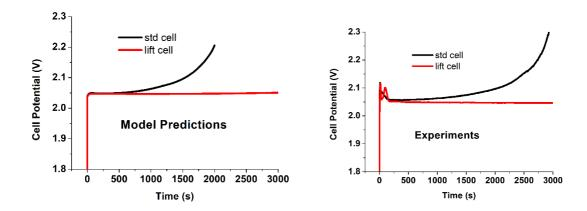
The figure above shows the model validation for charge performance in standard and lift cell design for natural convection case.
